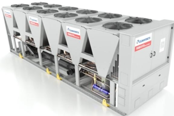
**Outdoor unit for the production of chilled water with semi-hermetic variable-speed screw compressors optimized for R134a, axial-flow fans, micro-channel full-aluminum condensing coils, single-pass shell and tubes evaporator designed by Mitsubishi Electric Hydraulics & IT Cooling Systems S.p.A. and electronic expansion valve.**
