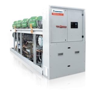
Indoor unit for the production of chilled water featuring centrifugal compressors oil-free, with refrigerant HFO (1234-ze), electronic regulation valve, shell and tube condenser and shell and tube flooded evaporator. Base and supporting structure and panels are of galvanized epoxy powder coated steel with increased thickness.
