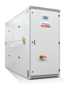
Water to water indoor unit for the production of chilled water with hermetic rotary Scroll compressors, braze-welded plate-type exchanger and electronic expansion valve. Basement and frame in hot-galvanised shaped sheet steel with a suitable thickness. All parts polyester-powder painted to assure total weather resistance, RAL 7035.
