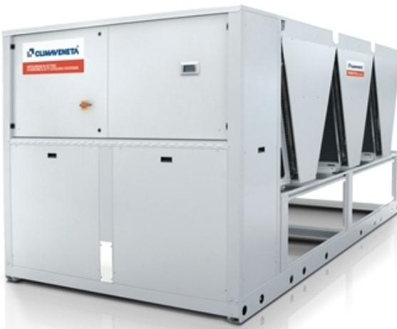
**Outdoor unit for the production of chilled water with hermetic rotary Scroll compressors, ozone-friendly refrigerant R410A, axial-flow fans, shell and tubes heat exchanger, micro-channel full-aluminum air coils and thermostatic or electronic expansion valve, according to the model. The range is composed by units equipped with four compressors in tandem configuration on two independent refrigeration circuits.**
