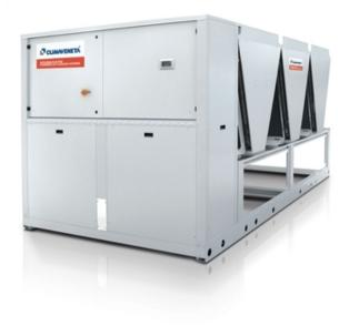
Outdoor unit for the production of chilled water with hermetic rotary Scroll compressors, ozone-friendly refrigerant R410A, axial-flow fans, braze-welded plate-type heat exchanger, micro-channel full-aluminum air coils and thermostatic expansion valve. The range is composed by units equipped with four compressors in tandem configuration on two independent refrigeration circuits.
