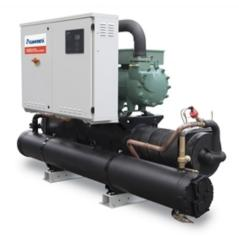
Indoor unit for the production of chilled water featuring semihermetic screw compressors optimized to operate with low compression ratio and R513A, shell and tubes evaporator designed by Mitsubishi Electric Hydronics & IT Cooling Systems S.p.A. and shell and tube condenser and electronic expansion valve.
