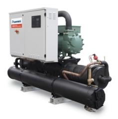
Indoor unit for the production of chilled water featuring semihermetic screw compressors optimized to operate with low compression ratio and R134a, shell and tubes evaporator designed by Mitsubishi Electric Hydronics & IT Cooling Systems S.p.A. and shell and tube condenser and electronic expansion valve.
