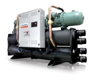
Single circuit indoor unit for the production of chilled water, with fixed speed and variable speed (Inverter Driven) screw compressors optimized for R513A, electronic expansion valve, high performing shell and tube condenser and shell and tube flooded evaporator, both designed and produced by Mitsubishi Electric Hydronics & IT Cooling Systems S.p.A. These technological solutions enhance the EER values over 5.7 at Eurovent standard conditions.
