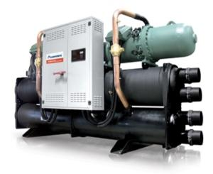
Single circuit indoor unit for the production of chilled water, with fixed speed and variable speed (Inverter Driven) screw compressors optimized for R134a, electronic expansion valve, high performing shell and tube condenser and shell and tube flooded evaporator, both designed and produced by Mitsubishi Electric Hydronics & IT Cooling Systems S.p.A. These technological solutions enhance the EER values over 5,7 at Eurovent standard conditions.
